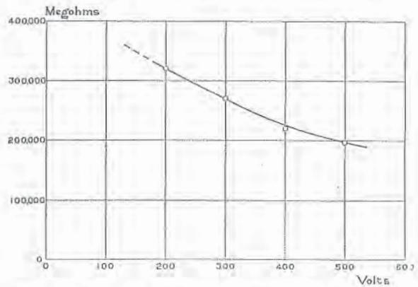
FIG. 19.—The same test-piece as in Fig. 18 tested 24 hours after being dried in an oven. Note: One hour after removal from the oven this test-piece had a resistance of 1,300,000 megohms at 500 volts.
