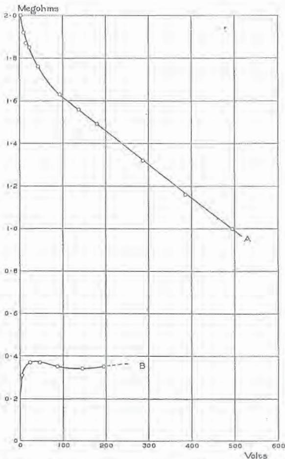
FIG. 4.—Insulation resistance of Lighting Circuits : A, in dry weather ; B, in very wet weather.
